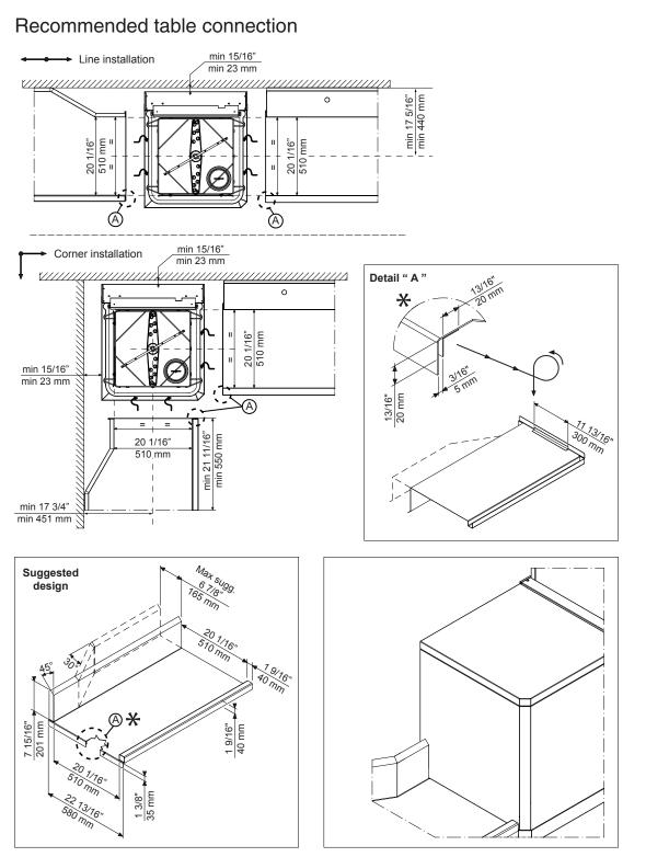
All tables must be connected to the dishwashing units according to local regulations and industry standards which may differ from the recommendations herein suggested. Electrolux Professional is not liable for any failure in complying with local design standards.
